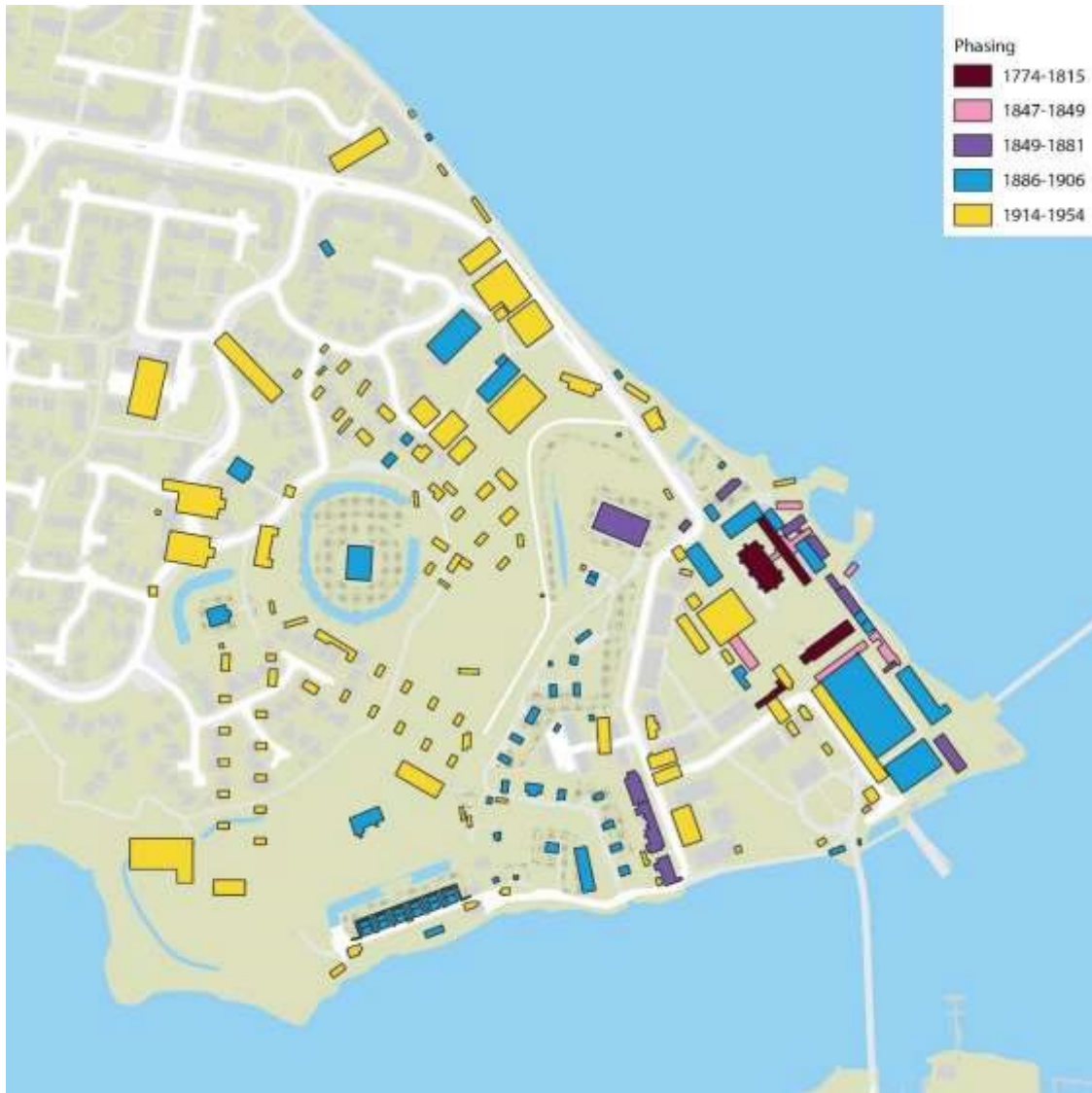
Figure 48 Phasing diagram of Priddy's Hard, showing extant depot buildings in 1988, the year of closure. Each building is coloured according to the phase of development in which it was constructed.
