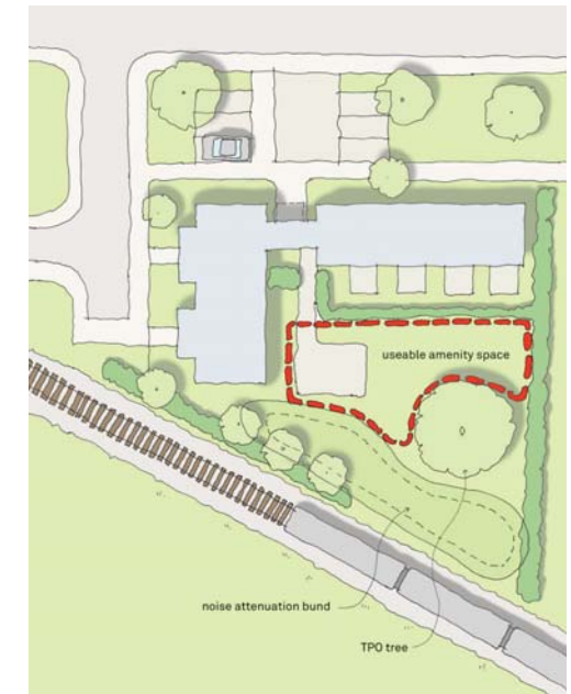
Fig 41: Useable amenity space excludes narrow strips of land and areas subject to excessive shading and noise attenuation bunds
