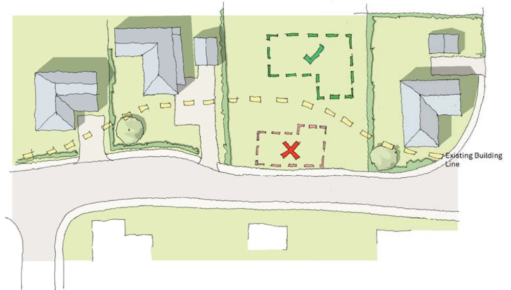
Fig 13: Existing building lines should be the starting point for continuing the urban grain with a new development
