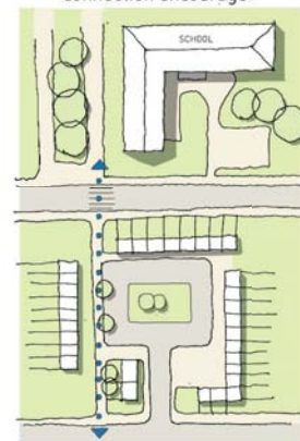
Fig 6: Alternative pedestrian and cycles accesses should be preserved or created where possible, to increase accessibility to important facilities
