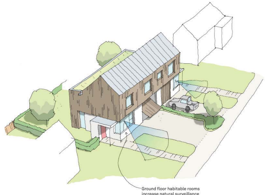
Fig 48: Properties with integral garages benefit from windows to habitable rooms at ground level to maximise the opportunities for surveillance
