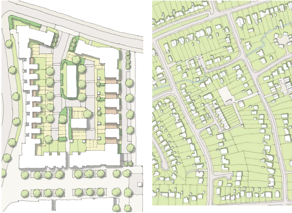
Fig 28: A typical suburban perimeter block layout (a) and a generic mixed use urban perimeter block (b)
