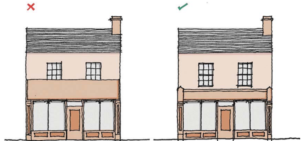
Fig 82: A proportionate fascia versus a fascia which dominates the building and obscures architectural features
