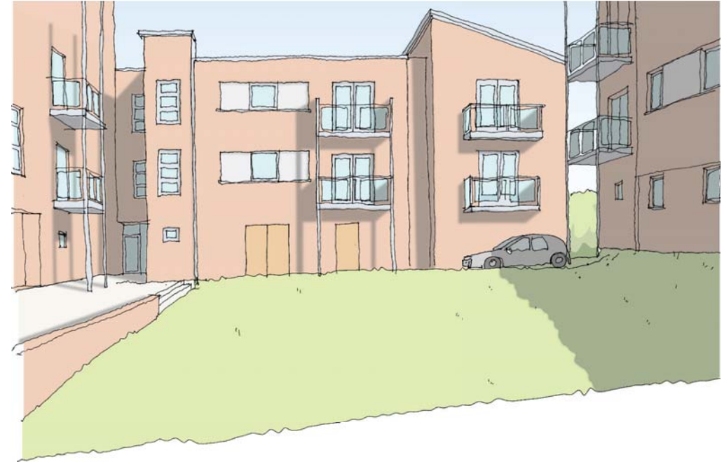
Fig 16: Inappropriate building mass can make an open space and gardens feel claustrophobic and uncomfortable for the users
