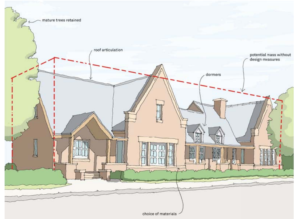
Fig 18: The perceived mass of a building can be reduced by a variety of design measures
