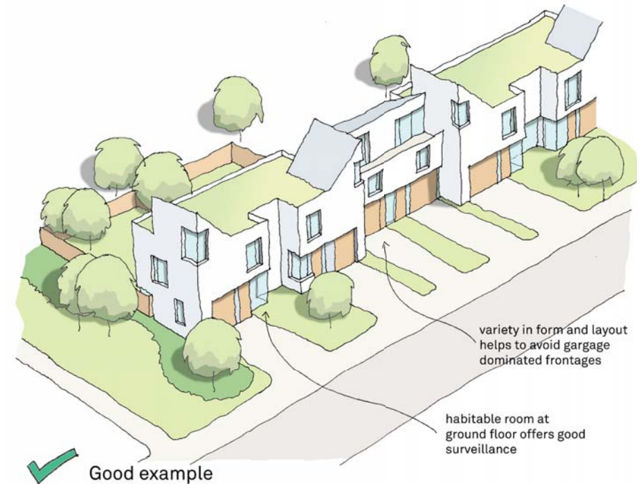
Fig 61: Good example of in-curtilage garages
