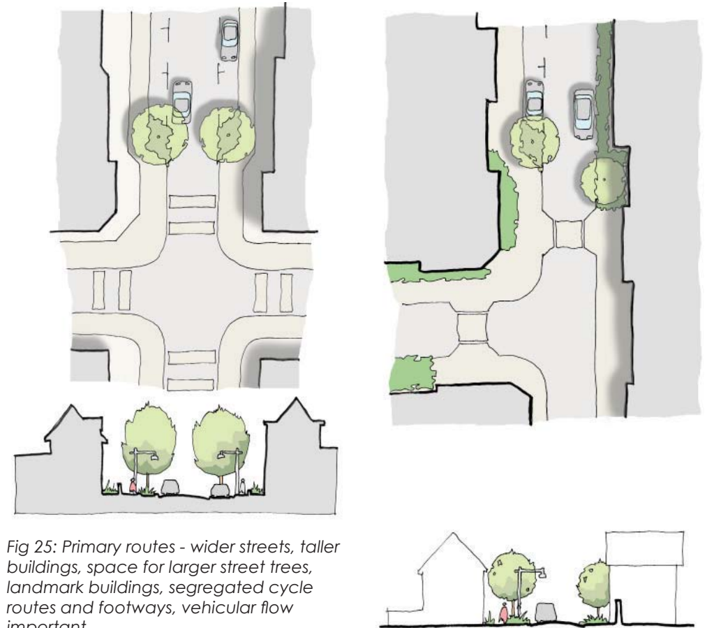
Fig 26: Secondary routes - modest street widths, smaller buildings, mostly smaller street trees and designed space for larger street trees, local landmark buildings, cycle routes and footways may not be segregated, on street car parking
