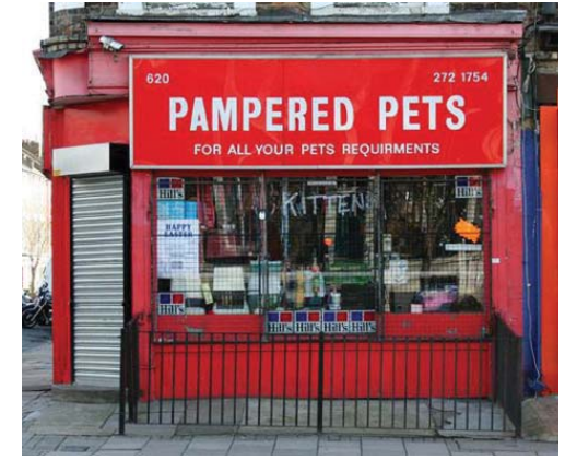
Fig 85: Fascia is disproportionate to building and shopfront design (Photo credit – Emily Webber)
